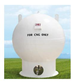
ASME Spheres –48" Inside Diameter. Manufactured and stamped per ASME Code, Section VIII, Division 2. Each sphere comes complete with one (1) 1" relief valve with isolation and bleed block, one (1) 1" service valve, and one (1) 1/2" drain valve. Each sphere is mounted on a skirt with a base plate, sand blasted, primed, top coated white, and stenciled "FOR CNG ONLY."
