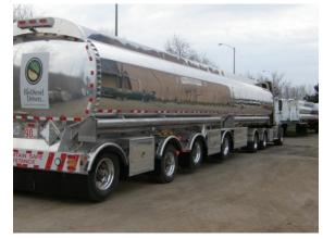
FIBA Canning Trailer with Almac tank: 18,000 / 15,000 / 15,000 / 15,000 litres; **Total capacity – 63,000** litres.
